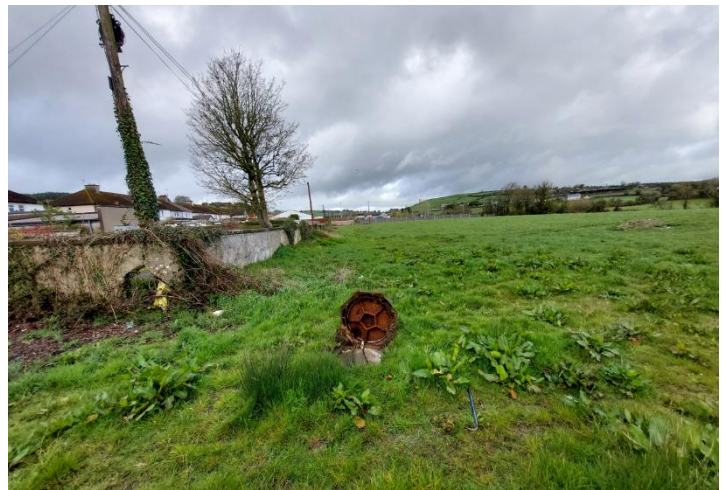
Photo 4: View looking Westwards, showing greenfield site and existing wall behind St. Bridget's Villas rear laneway. An existing Uisce Eireann sewer line is located behind this wall (within the site/field), a 6m wayleave/buffer is required which will extent from this wall out towards the site/field (no development is proposed over this wayleave).
